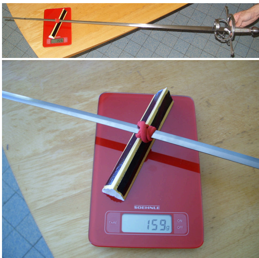
Figure 6: Weighing the blade mass. The sword rests horizontally on the finger at the handle-cross junction and on the support and scales at the center of oscillation, marked by the hair tie.
