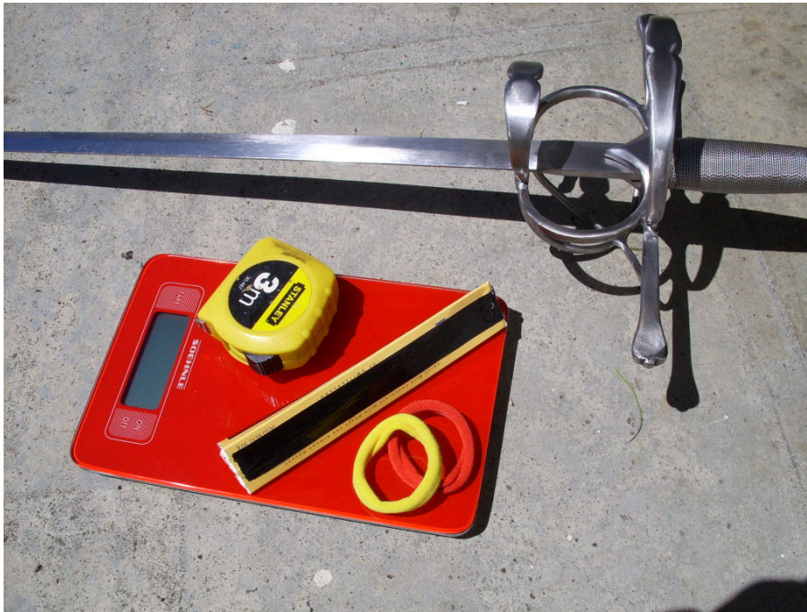
Figure 4: The tools used for the measure of the dynamic properties of swords: scales, tape ruler, hair ties, supporting objects. And of course the sword...
